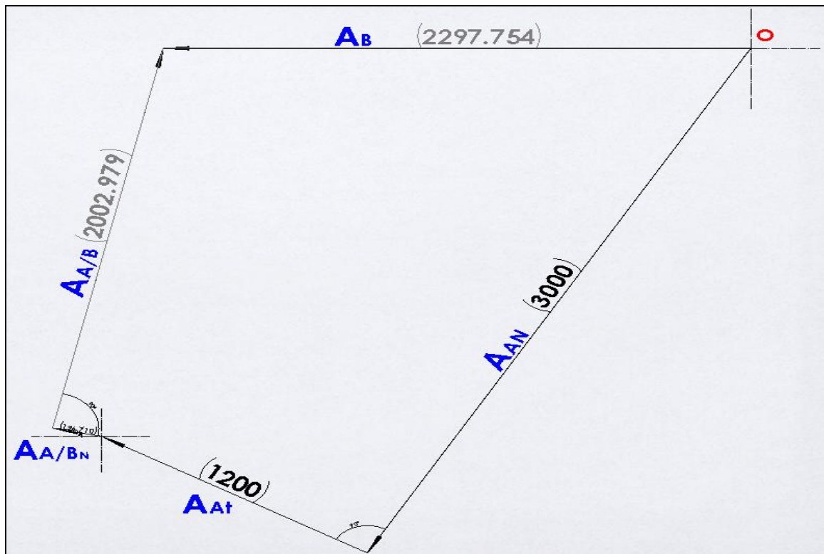
Figure 5: Acceleration diagram (60 degrees)
